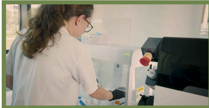
This type mass spectrometry (ICP-MS) uses inductively coupled plasma which atomizes and ionizes the sample in order to detect amounts of metals or non-metals in a the range of part per trillion.
